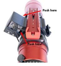
• While keeping a small amount of force on the front body of the Q-Focuser, secure the Q-Focuser to the bracket by fully tightening the four M3 screws. The belt should be taut but not rigid.
