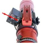
• Slip the belt over the telescope GT2 gear and the Q-Focuser pulley.
