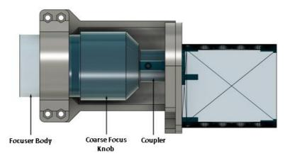
Warning: Do not attempt to remove the coarse focus knob. Meade used a thread locker on the screws and any attempt to remove the coarse knob screws could damage the screw heads.
