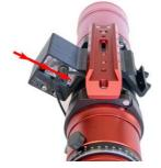
• Slip the belt over the telescope GT2 gear and the EAF pulley.
