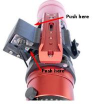
• While keeping a small amount of force on the front body of the EAF, secure the EAF to the bracket by fully tightening the two M4x10mm pan head screws. The belt should be taut but not rigid.
